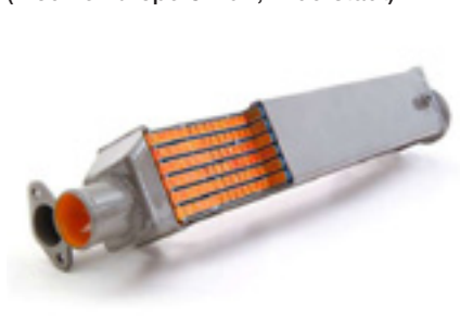
Exhaust gas heat exchanger made of stainless steel with nickel base brazing material, brazed in a vacuum, high temperature procedure (pattern) (Modine Europe GmbH, Filderstadt)
