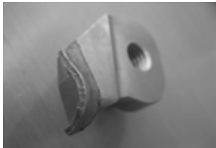
Brazed wear and tear protective layer on peeling tool (Euromat GmbH, Baesweiler)
