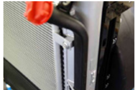
Heat exchanger for trucks in module aluminium sheeting, CAB brazed (Modine Europe GmbH, Filderstadt)
