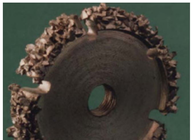
Specimen of an abrasive tool (Innobraze GmbH, Esslingen)
