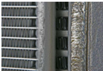
Welding and CAB brazing in heat exchangers, here truck charge air radiator and air conditioning capacitor (Modine Europe GmbH, Filderstadt)
