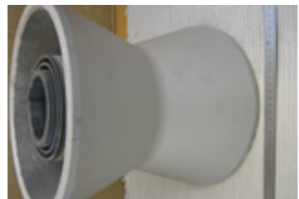
Brazed wear and tear protective layer on transport roller (Euromat GmbH, Baesweiler)
