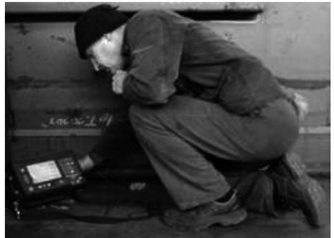
Ultra sound inspection of weld seams
