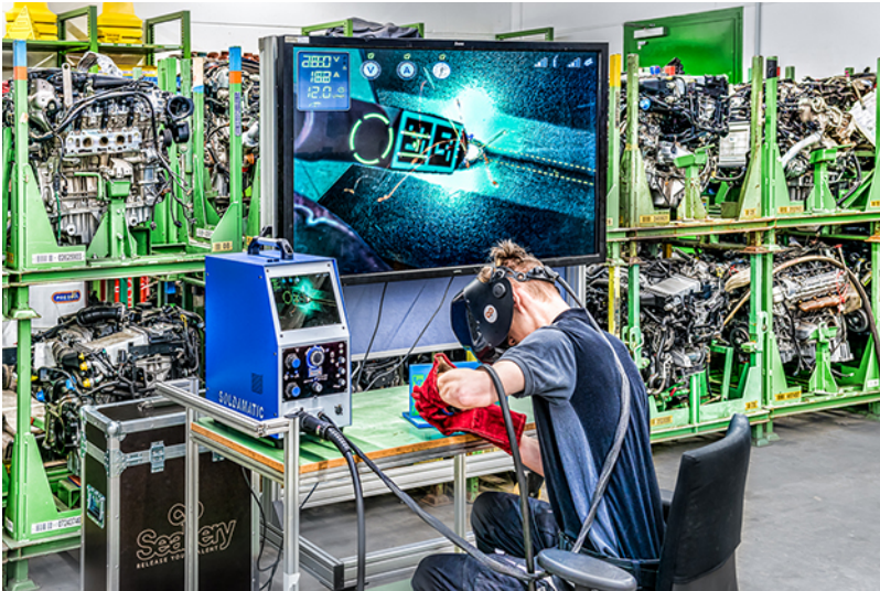
Welder in simulation-supported AR training with SOLDAMATIC.
